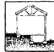
Treat each foundation separately and use the appropriate techniques for each foundation segment. Pay special attention to the points at which different foundation types join, because soil-gas entry routes exist in such locations. For an alternative, see page 43.
