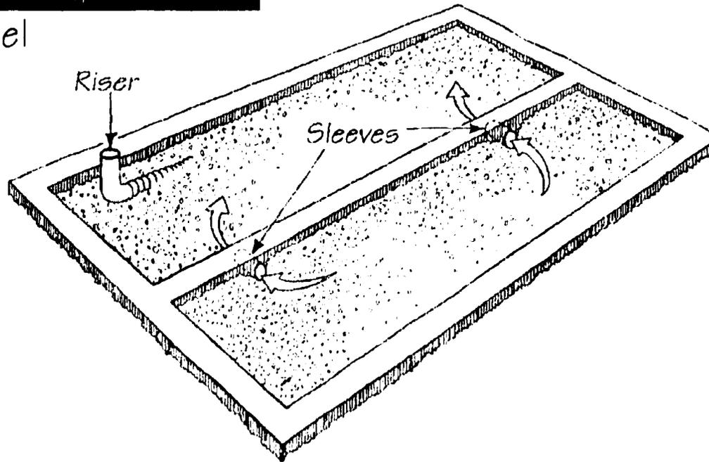
Place a uniform layer of clean aggregate under all concrete slabs or floor systems that directly contact the ground and are within the walls of the living spaces. Use a minimum 4-inch thick layer. The gravel should be about ½- to ¾-inch size. Smaller or fine gravel, or gravel that is not as uniform in size, will restrict air movement under the slab.
