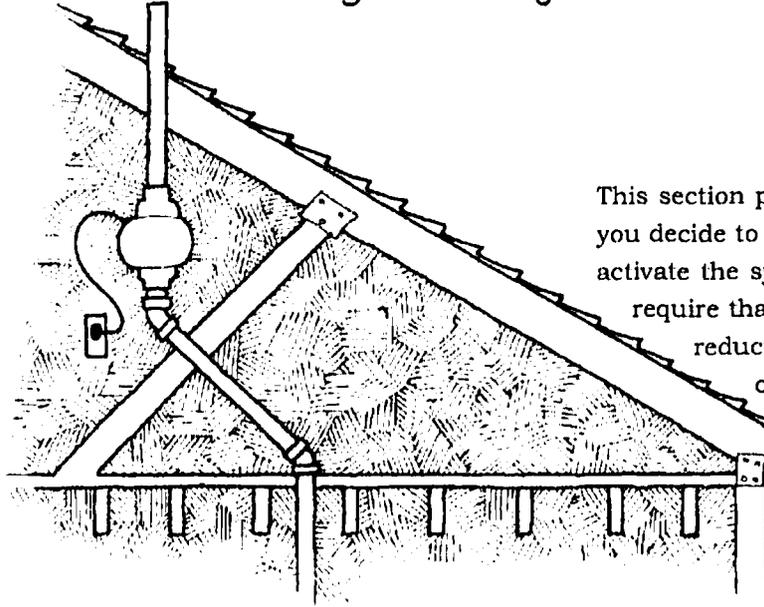
This section provides basic guidelines if you decide to install an in-line fan to activate the system. Some states require that in-line fans for radon reduction be installed by a certified radon mitigation contractor. Call your state radon contact for a list of certified contractors (see Appendix D for a list of phone numbers).
